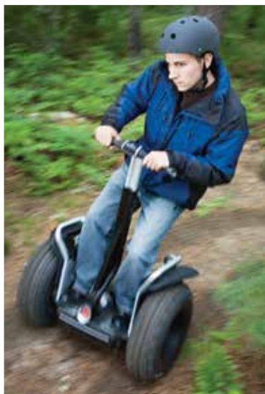
A Segway® personal transporter is an example of two-wheeled balancing.
