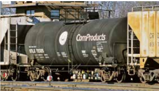
Tank cars carry liquids, mostly petroleum products such as fuel oil and petrochemicals, and liquids like vegetable oil, and are sometimes pressurized. Some tank cars have special linings to contain hazardous chemicals.
