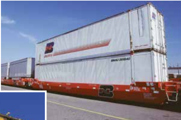
Highway truck trailers are carried in piggyback formation on flatcars, much like the way circus and farm wagon trains had traveled in earlier years.
