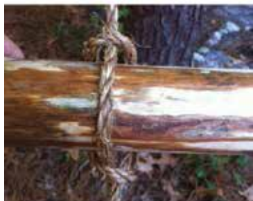
Adjust the rung and tighten the hitch.
