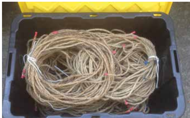
Lashing ropes, stored safely and conveniently. Note the color-coded tips representing each rope's length.
