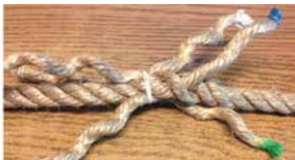
Short splice on a rope grommet
