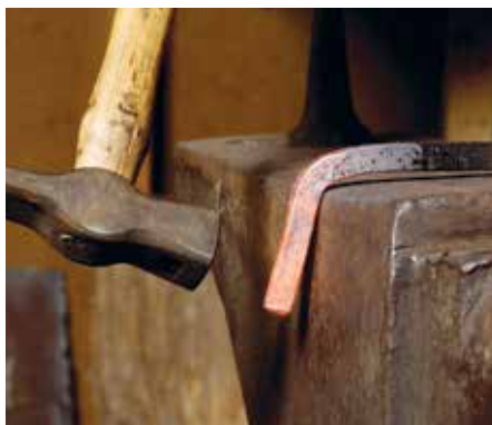
Bending steel over the edge of the anvil creates L-shaped bends.
