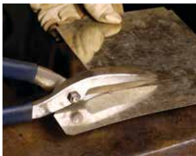
To cut a hole in sheet metal, first use a hollow punch to make a small hole inside the diameter of what will become the large hole. Then insert the tip of the snips into the punched hole. Cut in a circular pattern until the layout line is reached. Follow the layout line to complete the cut.
