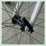
Three types of hubs and axles are used for wheels. Some bikes have solid axles with hex nuts on their ends to keep them tight on the forks or dropouts. Quick-release hubs have a hollow axle through which a rod passes, permitting the rapid installation and removal of a wheel. Many bikes now use thru axles where a large bolt passes through the hub and screws into one side of the fork or dropout; the bolt is loosened or tightened with an attached lever or with a hex wrench.
