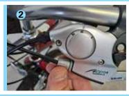
2. If the brake lever moves more than halfway toward the handlebar, add tension to the brake cable. If pads engage immediately when you pull the lever, the cable is too tight. Back out the barrel adjuster at the brake lever to allow for later adjustment.
