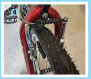
There should be an equal space between the rim and pads on each side.
