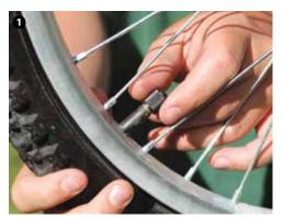
**Step 1**—First, check to see if the reason for the flat is the valve. The core in a Schrader stem can be tightened with a special cap or valve core wrench, but tubes with Presta stems must be replaced.
