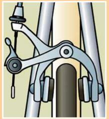
After the brakes are centered, check the whole brake system by squeezing the lever several times to see that the parts work promptly, nothing slips, and everything returns to a natural position when the levers are released.
