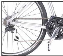
A good time to inspect the drive train and the rest of the bike for worn or broken parts is right after it has been cleaned.
