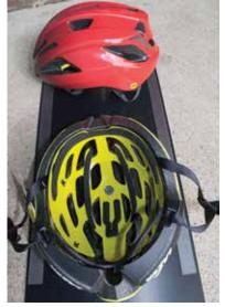
Helmet technology aims to reduce rotational force, which correlates to how much the brain moves inside the skull during an impact. The two most common are Multidirectional Impact Protection System (MIPS) and WaveCel. A MIPS helmet has an inner liner that absorbs rotational forces while the foam outer layer absorbs impacts.
