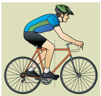
On a road bike, the handlebar ends should be tilted up or down so they are parallel to the ground. If the handlebars are in the correct position, your back should be at a 45-degree angle when you are riding. (This angle is a suggested guideline; your personal preference may vary.) If not, you may have to change to a different size handlebar stem or adjust the height of the bars.
