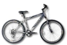
The features that make MTBs ideal for rugged ground also make them less suitable for longer trips on paved roads.
