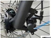
Barrel adjuster on cable disc brake
