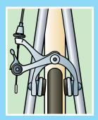
The front edge of the brake pad should be "toed in" so it contacts the rim slightly before the rear edge. Gently bend the flat surfaces of side-pull brake arms, or adjust the washers on centerpull brakes. Once the brakes are aligned with the rim, have a friend hold the brake pads (or use a tool or a piece of string), then tighten their bolts to secure them. You also do this to fix squeaky brakes.
