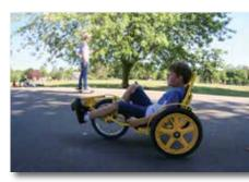
A recumbent bicycle or tricycle may be easier for a physically challenged person to power. Some are adapted so that they can be pedaled with the hands rather than the feet.
