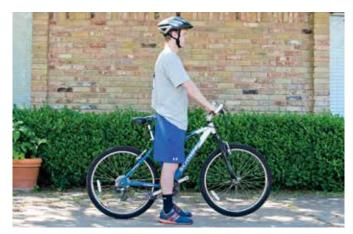
Check the fit by straddling the top tube and lifting the handlebars until the top tube reaches your crotch. On a road bike with a horizontal top tube, there should be 1 inch of clearance; for a road bike with a sloping top tube, look for 2 or more inches of clearance. For a mountain bike, there should be 2 to 4 inches of clearance.
