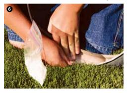
**Step 6**—To make remounting the tire easier, use talcum powder to coat the inside of the tire, the bead of the casing, and the tube.
