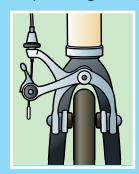
Loosen the anchor bolt or quick release (shown here). On side-pull brakes, this bolt is on the arm. On center-pull brakes, this bolt is on the bridge-wire hook. The main brake cable is now free to move, and you can adjust the brake pads so that they are aligned with the side of the rim when moved against the rim.
