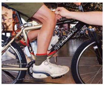
Some saddles can be adjusted forward or backward. If your saddle has this feature, do the following: Put the right pedal in the 3 o'clock position and center the ball of your right foot on the pedal axle. Hang a weighted string next to the bottom of your right kneecap. The string should pass through the center of the pedal axle. If the string is behind the axle, move the saddle forward. If it is in front, move the saddle backward. Next, make sure the saddle is level and not tilted up or down.
