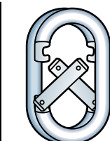
Always use nonlocking carabiners in pairs, with the gates of the carabiners reversed.
